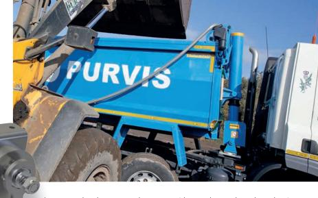
then carry the sheet up and over the load, before being lowered into its closed position at the rear. When retracting the sheet back to behind the body's headboard, tension is then built up in the springs as the sheet is pulled forwards and back into its stored position.
